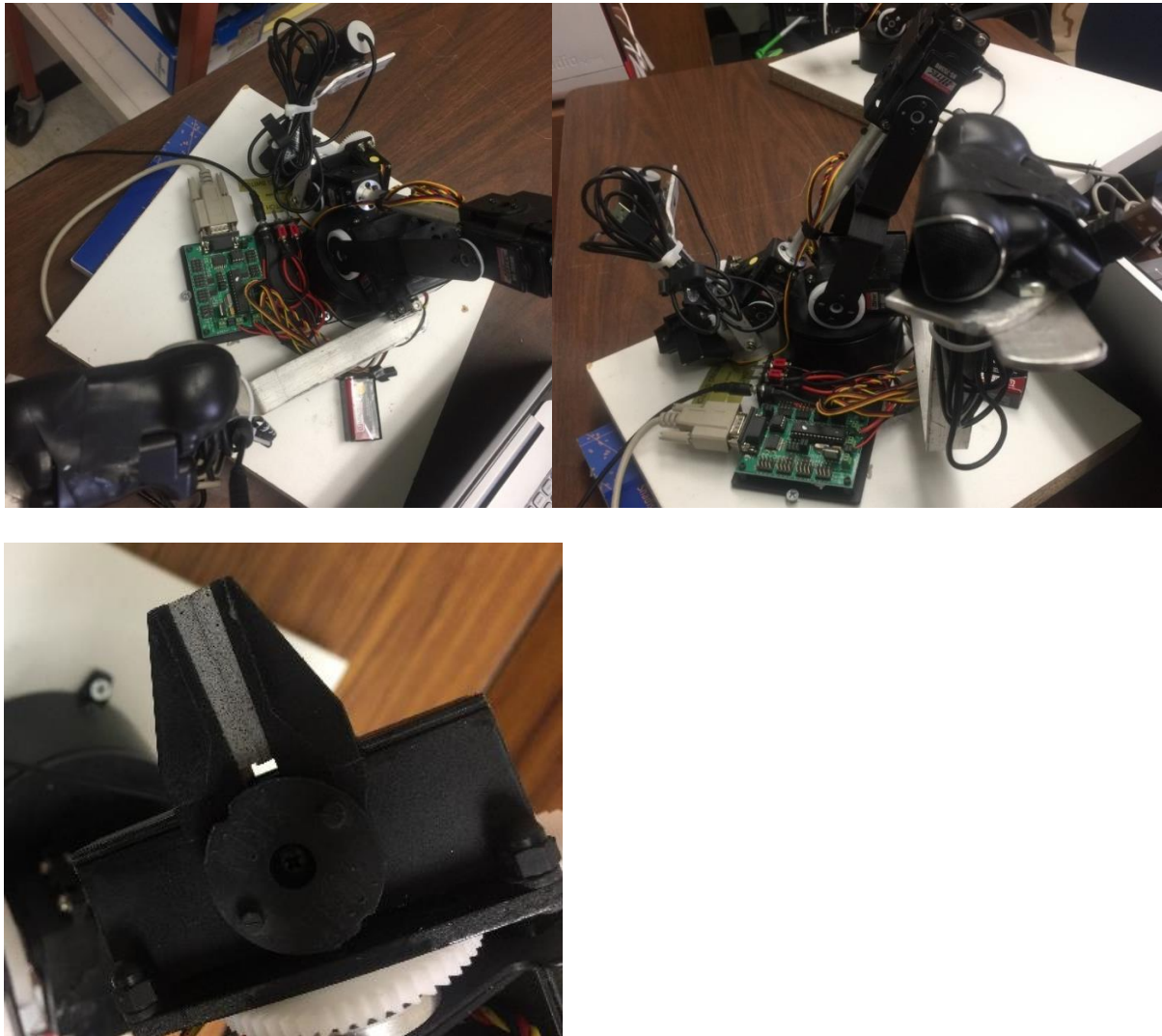
Figure 8. The Karlsson Robotics Lynxmotion ALD5D 4 degrees of freedom robotic arm used in the experiment.
