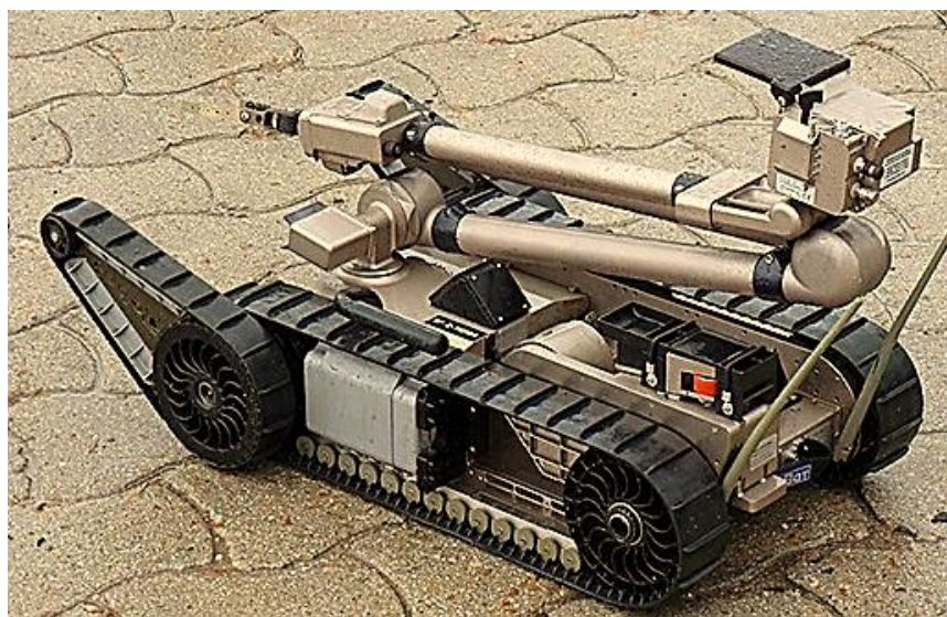
Figure 1. Image of iRobot 510 PackBot used to disassemble IEDs (Army Technology, 2018).
